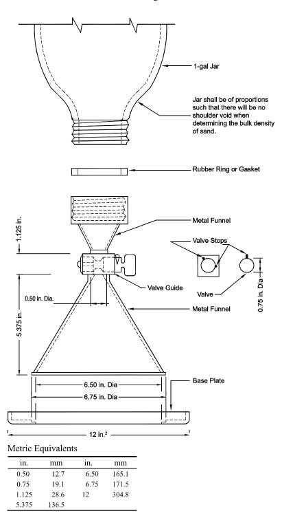
Figure 1—Density Apparatus
